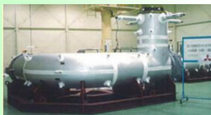
Concentric hot gas duct
